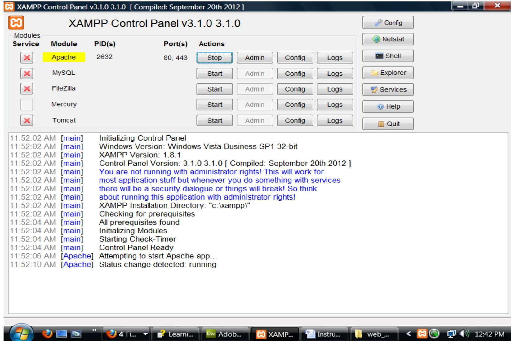
Fig 1.1 XAMPP control panel from where we can start or stop the various services provided by different modules.
